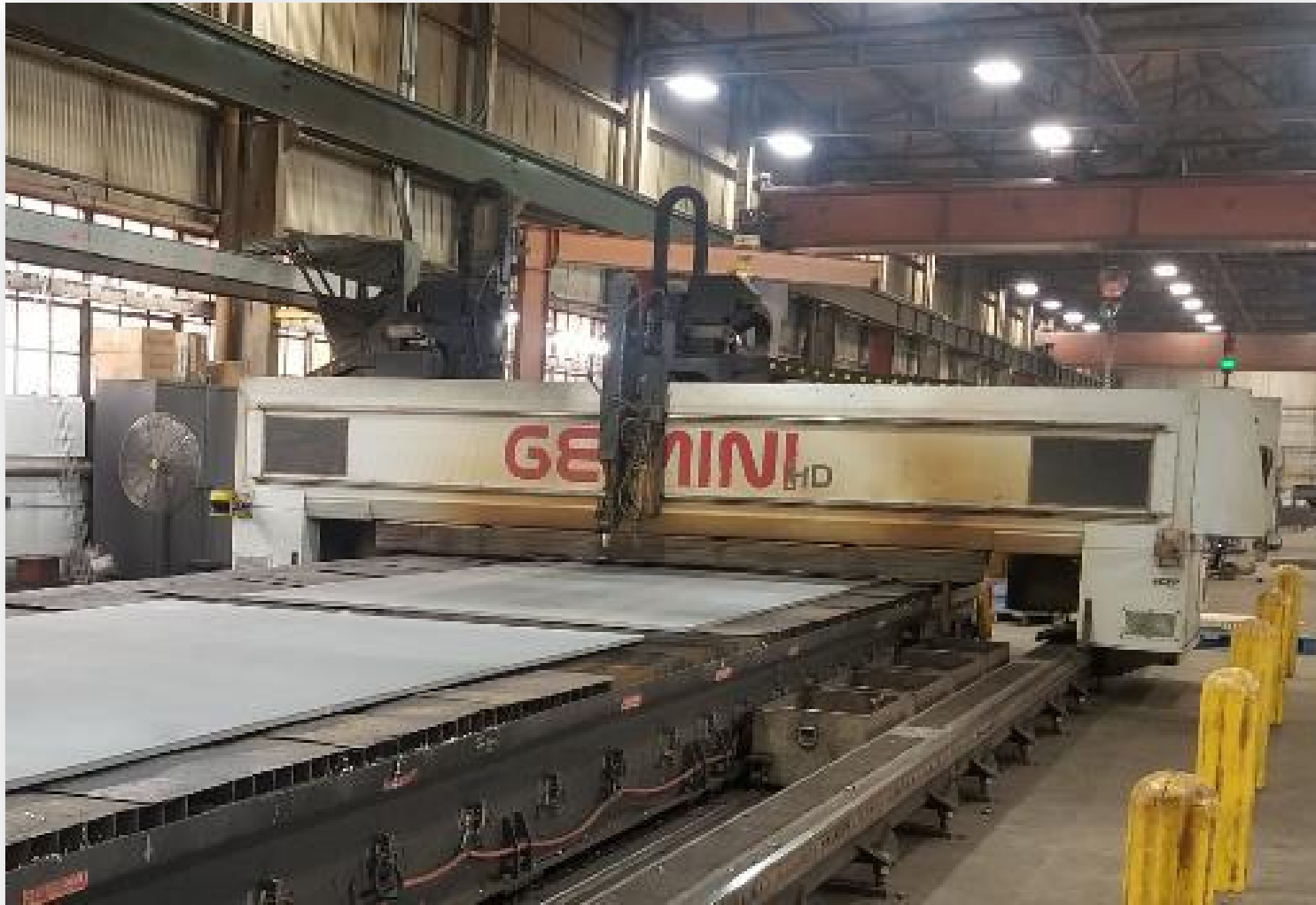
This machine does CNC cutting and drilling
